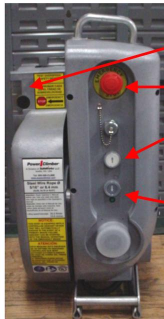
Overspeed Brake Test Button
