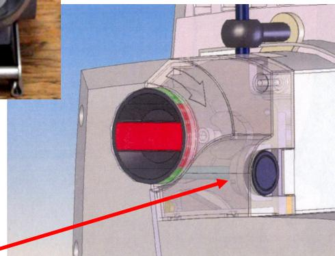
**Overspeed Brake Test Button**
